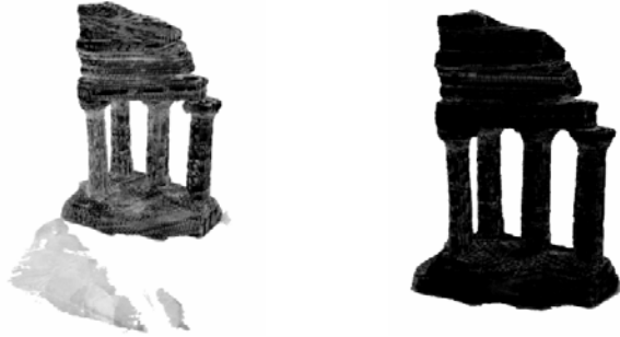
Fig. 3. Reconstruction after 16 random sparse views (left) and after 28 views (16 plus 12 chosen to reduce uncertainty; right). Gray points identify uncertainty, black points identify actual voxels and transparent points are the eliminated voxels.
