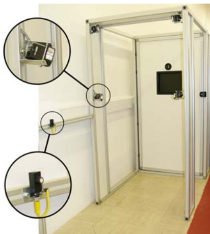
Fig. 1. Photograph of the geometry capture device. One of the light sources and an ultrasound trigger are shown to the left. The camera is located on the back panel.
