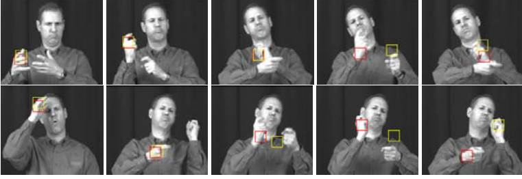
Fig. 4. Comparison of vision-based tracking (yellow) and joint vision- and stereo-vision-based tracking (red) of the dominant hand performing rotating and overlapping hand movements (first row) and fast asynchronous upward and downward movements (second row)
